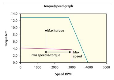
Max torque = 10Nm: Max speed = 2900 rms torque = 3Nm: rms speed = 1500
