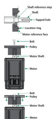
Screw the bolt into the tapped hole of the shaft and, while holding the pulley, use it to push the pulley down and pull the shaft through at the same time.
