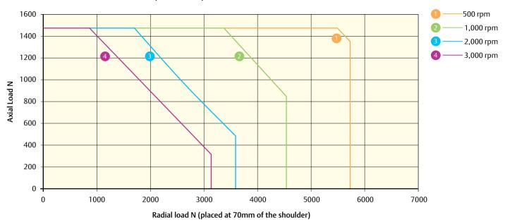
$250U2\,L_{10(h)}$  Bearing life for 20,000 hours (reliability 90%, load factor of 1). Do not exceed a maximum axial load of 1450 N
