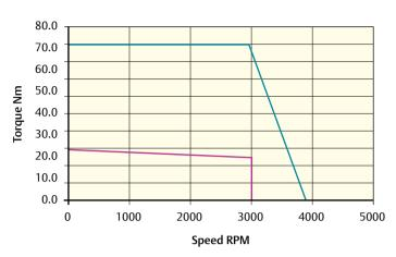
Peak torque (Nm) = 70.20 Stall torque (Nm) = 29.5 Rated torque (Nm) = 25.0
