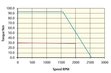
Peak torque (Nm) = 28.2 Stall torque (Nm) = 9.6 Rated torque (Nm) = 9.3 Peak torque (Nm) = 93.3 Stall torque (Nm) = 31.1 Rated torque (Nm) = 28.4
