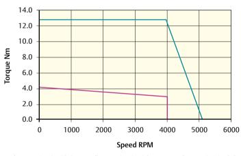
Peak torque (Nm) = 12.9 Stall torque (Nm) = 4.3 Rated torque (Nm) = 3.0
