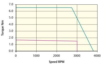
Peak torque (Nm) = **6.60** Stall torque (Nm) = **1.65**
