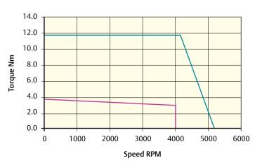
Peak torque (Nm) = 11.7 Stall torque (Nm) = 3.9 Rated torque (Nm) = 2.9
