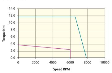
Peak torque (Nm) = 11.7 Stall torque (Nm) = 3.9 Rated torque (Nm) = 2.6
