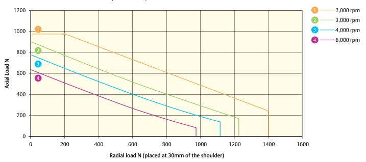
$142U2 L_{10(h)}$  Bearing life for 20,000 hours (reliability 90%, load factor of 1). Do not exceed a maximum axial load of 950 N
