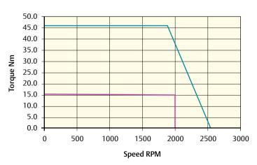
Peak torque (Nm) = 45.9 Stall torque (Nm) = 15.3 Rated torque (Nm) = 14.6
