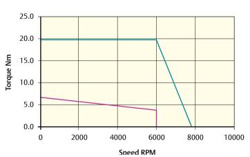
Peak torque (Nm) = 19.8 Stall torque (Nm) = 6.6
