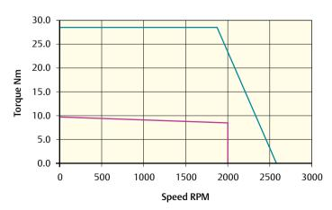
Peak torque (Nm) = 28.2 Stall torque (Nm) = 9.4 Rated torque (Nm) = 8.7
