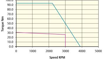
Peak torque (Nm) = 93.3 Stall torque (Nm) = 31.1 Rated torque (Nm) = 25.0
