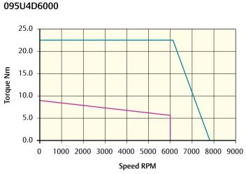
Peak torque (Nm) = 22.50 Stall torque (Nm) = 9.0 Rated torque (Nm) = 5.8
