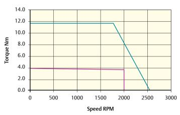
Peak torque (Nm) = 11.7 Stall torque (Nm) = 3.9 Rated torque (Nm) = 3.8
