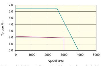
Peak torque (Nm) = **6.6** Stall torque (Nm) = **2.2** Rated torque (Nm) = **2.0**
