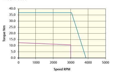
Peak torque (Nm) = 37.4 Stall torque (Nm) = 12.4 Rated torque (Nm) = 10.4
