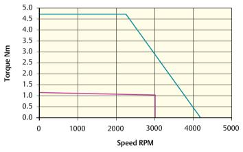
Peak torque (Nm) = 4.72 Stall torque (Nm) = 1.18 Rated torque (Nm) = 1.05
