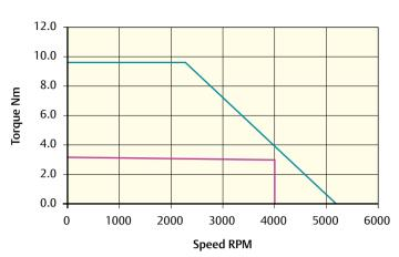
Peak torque (Nm) = **9.60** Stall torque (Nm) = **3.20** Rated torque (Nm) = **2.90**
