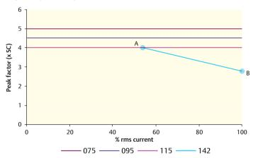
As shown above the 075 increases to 5 times, 095 increases to 4.5 times, the 115 increases to 4 times across the % rms current line and the 142 shows an increase to 4 times up until 57% dropping to 2.5 times at 100%.
