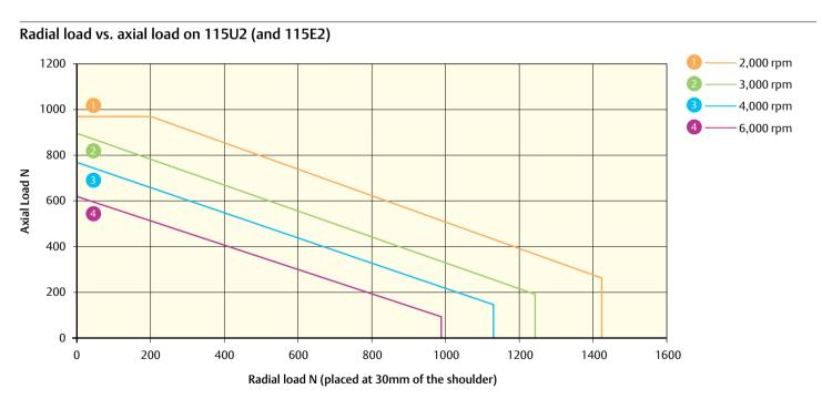
$115 U2\ L_{_{10(h)}} Bearing\ life\ for\ 20,000\ hours\ (reliability\ 90\%,\ load\ factor\ of\ 1).\ Do\ not\ exceed\ a\ maximum\ axial\ load\ of\ 950\ N$
