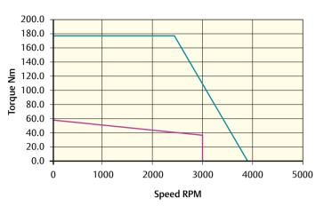
Peak torque (Nm) = 176.1 Stall torque (Nm) = 58.7 Rated torque (Nm) = 35.0
