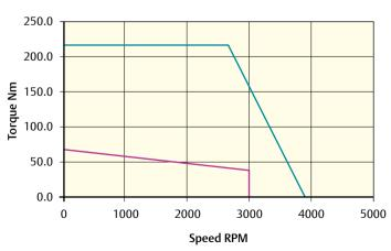
Peak torque (Nm) = 219.6 Stall torque (Nm) = 73.2 Rated torque (Nm) = 36.8
