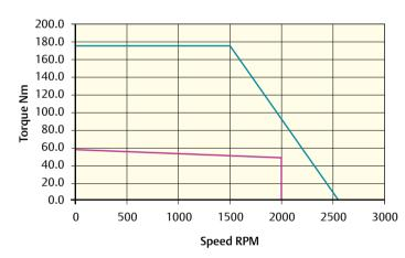
Peak torque (Nm) = 176.1 Stall torque (Nm) = 58.7 Rated torque (Nm) = 50.4
