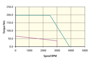
Peak torque (Nm) = 198.0 Stall torque (Nm) = 66.0 Rated torque (Nm) = 36.0
