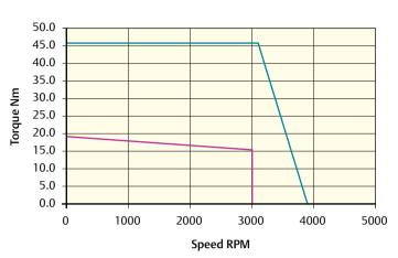
Peak torque (Nm) = 45.90 Stall torque (Nm) = 18.90 Rated torque (Nm) = 16.1
