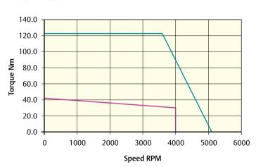
Peak torque (Nm) = 123.3 Stall torque (Nm) = 41.1 Rated torque (Nm) = 29.0
