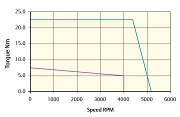
Peak torque (Nm) = 22.5 Stall torque (Nm) = 7.5 Rated torque (Nm) = 4.9
