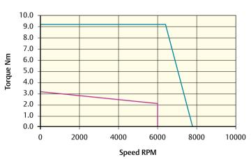
Peak torque (Nm) = 9.3 Stall torque (Nm) = 3.1 Rated torque (Nm) = 2.1
