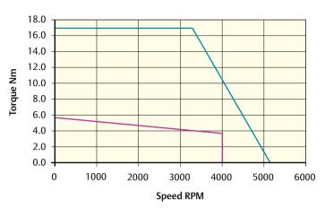
Peak torque (Nm) = 17.1 Stall torque (Nm) = 5.7 Rated torque (Nm) = 3.6
