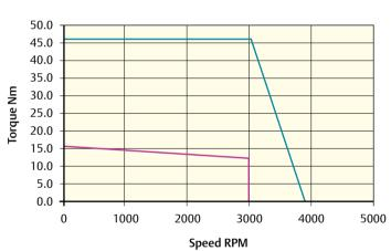
Stall torque (Nm) = 15.3 Rated torque (Nm) = 12.6 Peak torque (Nm) = 45.9
