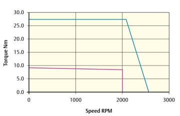
Peak torque (Nm) = 27.0 Stall torque (Nm) = 9.0 Rated torque (Nm) = 8.2
