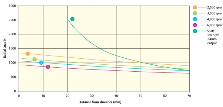
115UD L  $_{_{10(h)}}\mbox{Bearing}$  life for 20,000 hours (reliability 90%, load factor of 1)
