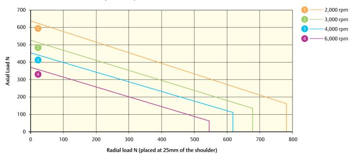
$95U2L_{10(h)}$  Bearing life for 20,000 hours (reliability 90%, load factor of 1). Do not exceed a maximum axial load of 850 N
