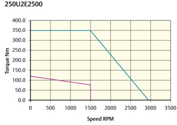
Peak torque (Nm) = 348.0 Stall torque (Nm) = 116.0 Rated torque (Nm) = 70.0
