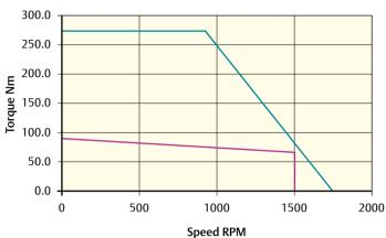
Peak torque (Nm) = 276.0 Stall torque (Nm) = 92.0 Rated torque (Nm) = 67.0
