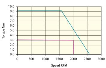
Peak torque (Nm) = 9.3 Stall torque (Nm) = 3.1 Rated torque (Nm) = 3.0
