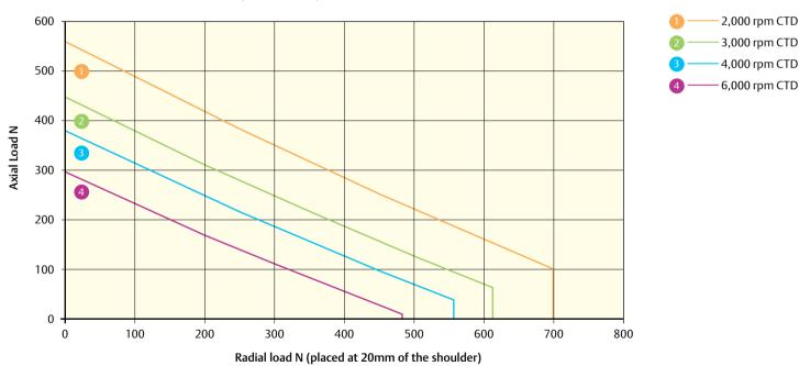
$067 UD\ L_{_{10(h)}} Bearing\ life\ for\ 20,000\ hours\ (reliability\ 90\%,\ load\ factor\ of\ 1).\ Do\ not\ exceed\ a\ maximum\ axial\ load\ of\ 650\ N$
