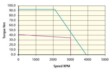
Peak torque (Nm) = **93.30** Stall torque (Nm) = **41.0** Rated torque (Nm) = **35.5**
