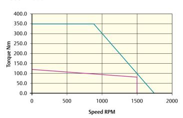
Peak torque (Nm) = 348.0 Stall torque (Nm) = 116.0 Rated torque (Nm) = 76.0
