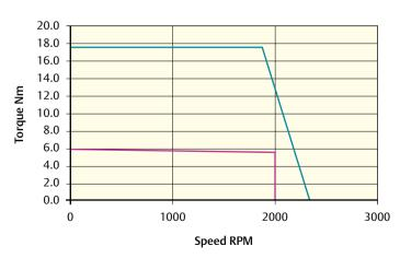
Peak torque (Nm) = 17.7 Stall torque (Nm) = 5.9 Rated torque (Nm) = 5.5
