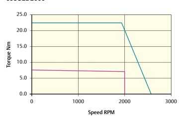
Peak torque (Nm) = 22.5 Stall torque (Nm) = 7.5 Rated torque (Nm) = 6.9
