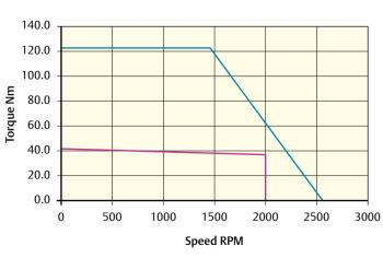
Peak torque (Nm) = 123.3 Stall torque (Nm) = 41.1 Rated torque (Nm) = 36.9
