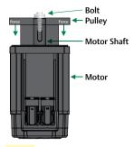
Once the bolt has bottomed out unscrew it and place another washer underneath. Continue this process until the pulley is squeezed home.
