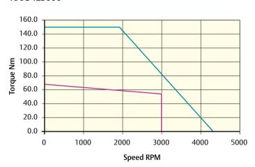
Peak torque (Nm) = 151.6 Stall torque (Nm) = 68.0 Rated torque (Nm) = 55.0
