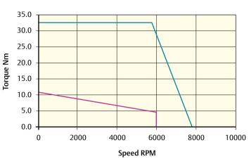
Peak torque (Nm) = 32.4 Stall torque (Nm) = 10.8 Rated torque (Nm) = 4.5
