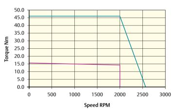
Peak torque (Nm) = 45.9 Stall torque (Nm) = 15.3 Rated torque (Nm) = 14.0
