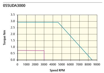
Peak torque (Nm) = 2.88 Stall torque (Nm) = 0.72 Rated torque (Nm) = 0.70
