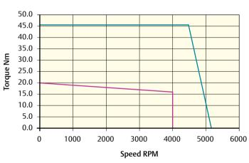
Peak torque (Nm) = 45.90 Stall torque (Nm) = 20.1 Rated torque (Nm) = 16.1
