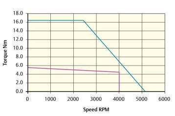
Peak torque (Nm) = 16.50 Stall torque (Nm) = 5.50 Rated torque (Nm) = 4.85 Peak torque (Nm) = 16.50 Stall torque (Nm) = 5.50 Rated torque (Nm) = 4.55
