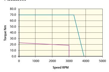
Peak torque (Nm) = 70.2 Stall torque (Nm) = 23.4 Rated torque (Nm) = 18.0
