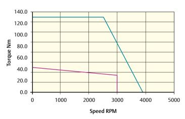
Peak torque (Nm) = 151.6 Stall torque (Nm) = 50.6 Rated torque (Nm) = 34.0
