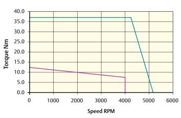
Peak torque (Nm) = 37.2 Stall torque (Nm) = 12.4 Rated torque (Nm) = 7.5
