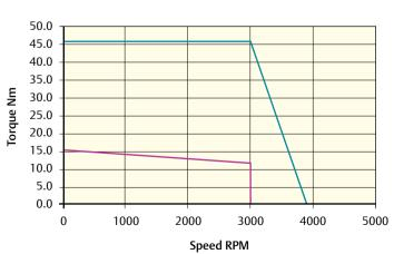
Peak torque (Nm) = 45.9 Stall torque (Nm) = 15.3 Rated torque (Nm) = 12.2
