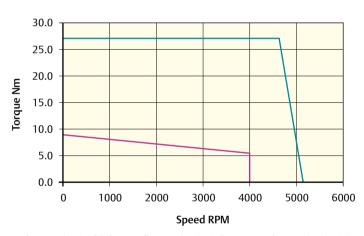
Peak torque (Nm) = 27.0 Stall torque (Nm) = 9.0 Rated torque (Nm) = 5.7
