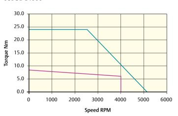
Peak torque (Nm) = 24.00 Stall torque (Nm) = 8.00 Rated torque (Nm) = 6.35
