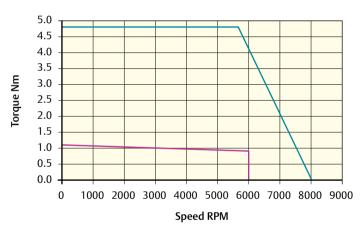
Peak torque (Nm) = 4.72 Stall torque (Nm) = 1.18 Rated torque (Nm) = 0.90
