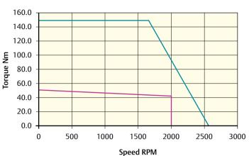
Peak torque (Nm) = **151.6** Stall torque (Nm) = **50.6** Rated torque (Nm) = **43.8**
