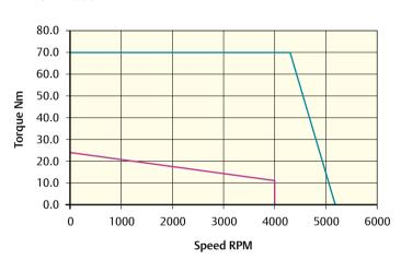
Peak torque (Nm) = 70.2 Stall torque (Nm) = 23.4 Rated torque (Nm) = 12.2
