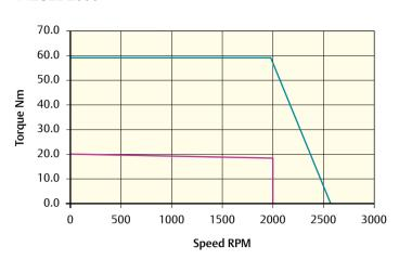
Peak torque (Nm) = 17.1 Stall torque (Nm) = 5.7 Rated torque (Nm) = 5.3 Peak torque (Nm) = 59.4 Stall torque (Nm) = 19.8 Rated torque (Nm) = 18.4
