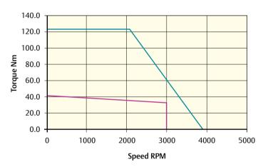
Peak torque (Nm) = 123.3 Stall torque (Nm) = 41.1 Rated torque (Nm) = 33.0
