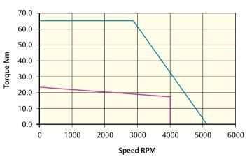
Peak torque (Nm) = 65.4 Stall torque (Nm) = 21.8 Rated torque (Nm) = 17.5
