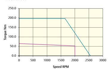
Peak torque (Nm) = 198.0 Stall torque (Nm) = 66.0 Rated torque (Nm) = 53.0
