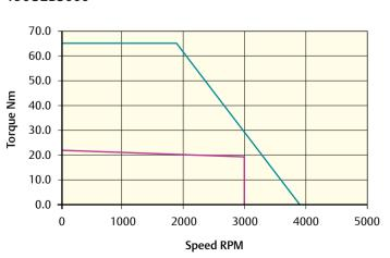
Peak torque (Nm) = 65.4 Stall torque (Nm) = 21.8 Rated torque (Nm) = 19.5
