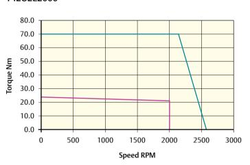
Peak torque (Nm) = 32.4 Stall torque (Nm) = 10.8 Rated torque (Nm) = 10.3 Peak torque (Nm) = 70.4 Stall torque (Nm) = 23.4 Rated torque (Nm) = 21.3
