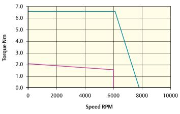
Peak torque (Nm) = 6.6 Stall torque (Nm) = 2.2 Rated torque (Nm) = 1.6
