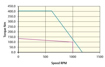
Peak torque (Nm) = 408.0 Stall torque (Nm) = 136.0 Rated torque (Nm) = 106.0
