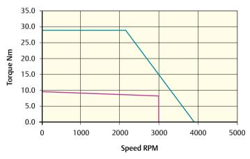
Peak torque (Nm) = 28.8 Stall torque (Nm) = 9.6 Rated torque (Nm) = 8.7
