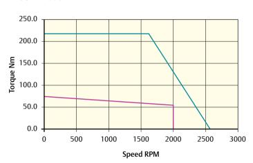
Peak torque (Nm) = 219.6 Stall torque (Nm) = 73.2 Rated torque (Nm) = 54.7
