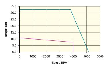
Peak torque (Nm) = 32.4 Stall torque (Nm) = 10.8 Rated torque (Nm) = 7.0
