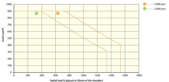
$190U2\ L_{10(h)}$  Bearing life for 20,000 hours (reliability 90%, load factor of 1). Do not exceed a maximum axial load of 900 N
